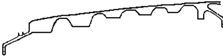
4.a - Ring Disk Drum Rotor Cross Section
